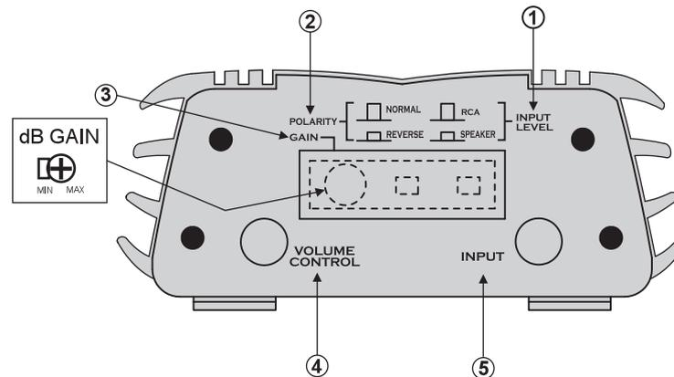
The switches and gain settings are located behind a watertight plug, which also lights up when the amplifier is on. Be sure to replace the plug when finished with adjustments.
