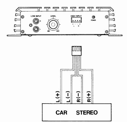
NOTE: THE ABOVE TYPES OF INPUT MUST BE USED INDEPENDENTLY. DO NOT CONNECT MORE THAN ONE INPUT AT THE SAME TIME.
