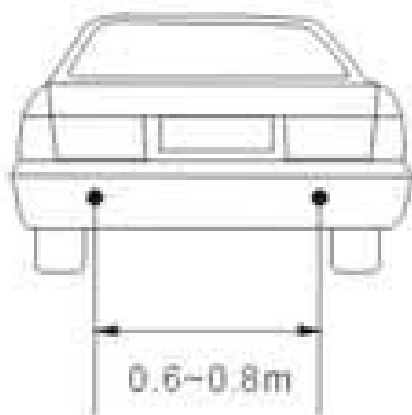
Install two sensor
